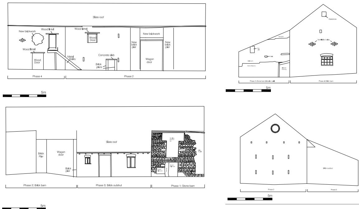
Fig. 2.34: Scale elevations of Building 4 (barn)
