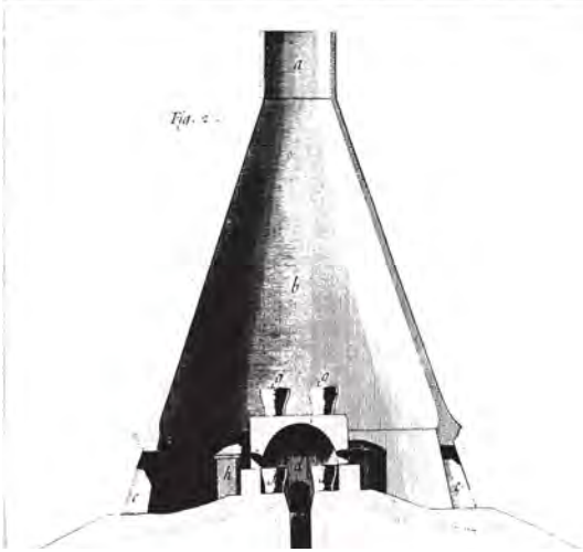
Fig. 2. Exterior view and section of an English-style cone glasshouse showing the large underground flue beneath the central furnace, from Diderot and D'Alembert's Encyclopédie, vol. 10, pl. 3
